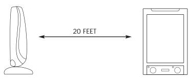
4. If you hear static or noise and the signal is not clear, set the FREQUENCY ADJUST knob to a new setting and then try to tune the speakers using the TUNING knob on each one. If you still do not get a clear signal, make certain that other devices that use RF frequencies such as cordless phones, cell phones and baby monitors are not operating in the home when you use your speakers as they can cause interference.
